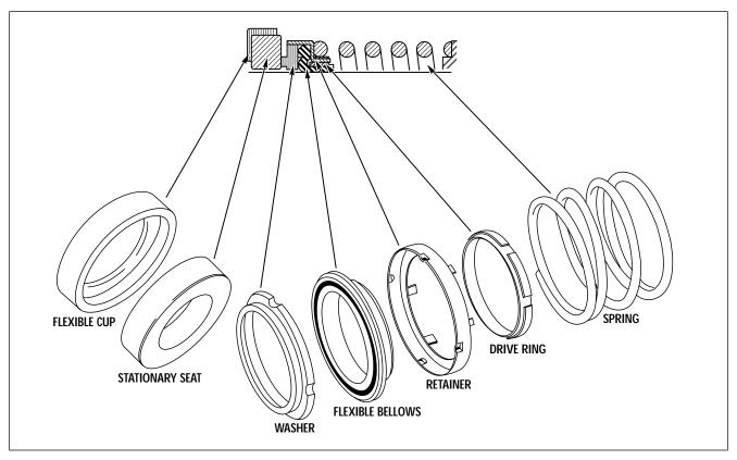
Figure 1. Mechanical Seal
